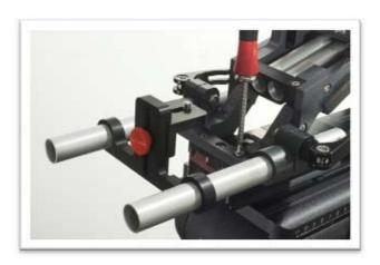
6) Screw the 1D camera table support on the extended camera table top
